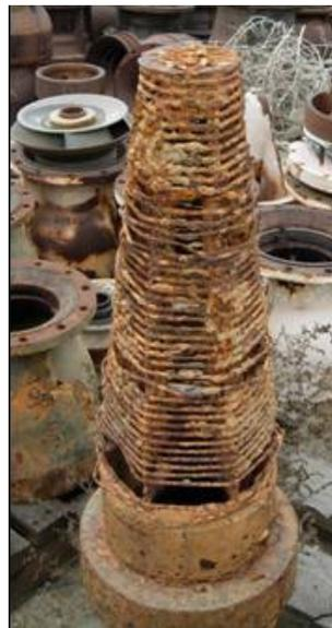
Figure 7. Corroded pump cone screen with missing sections.
