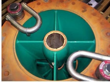
Figure 3. SK134 fusion bonded epoxy application.
