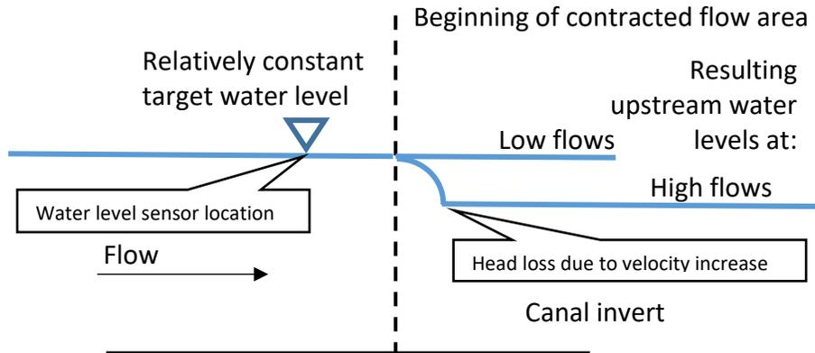
**Figure 4. Improved water level control in the pool with a different water level sensor location, with the same amount of head loss due to increased water velocity at an automatic upstream control gate (profile view)**
