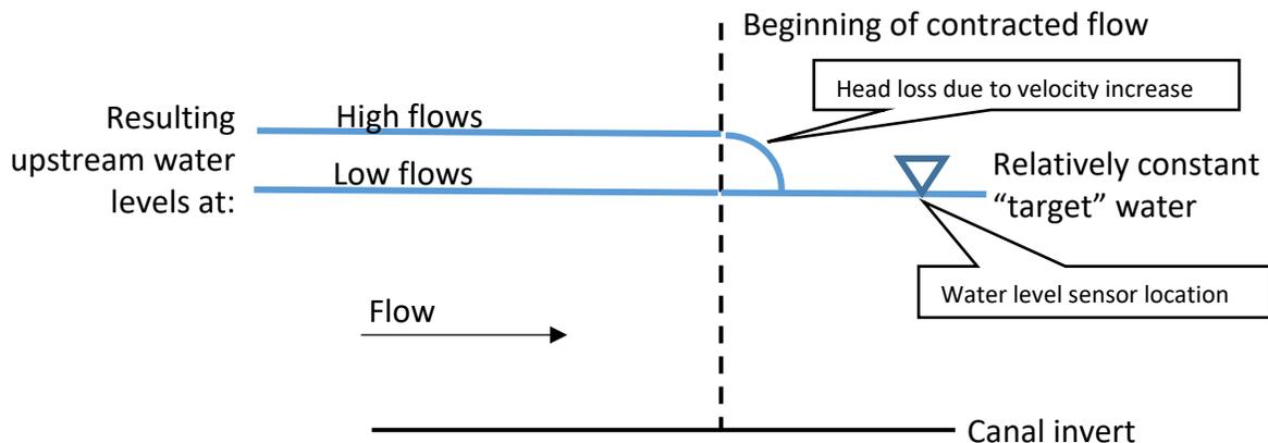
Figure 3. Potential fluctuations in the pool water level due to poor sensor location on a hypothetical automatic upstream control gate (profile view)
