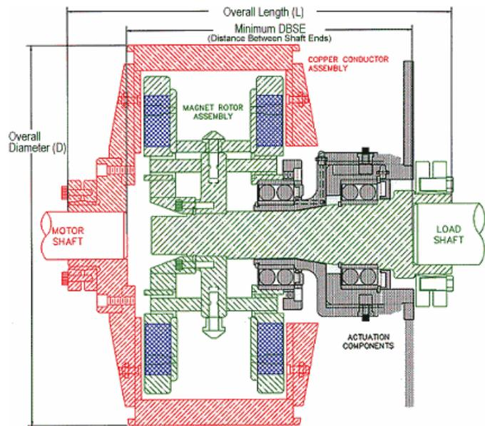
Figure 1. MagnaDrive Coupler Schematic
